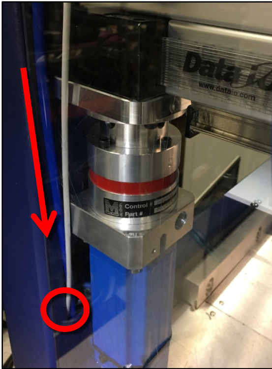
Route cables down through chassis opening/access cut-out.
